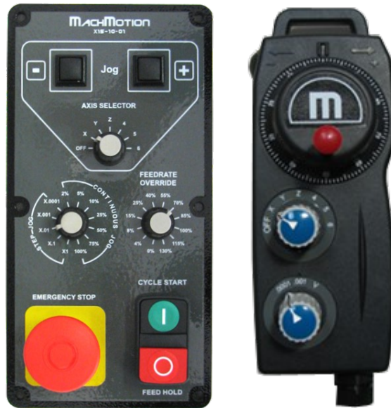
Figure 3-26: Control panel and pendant examples
